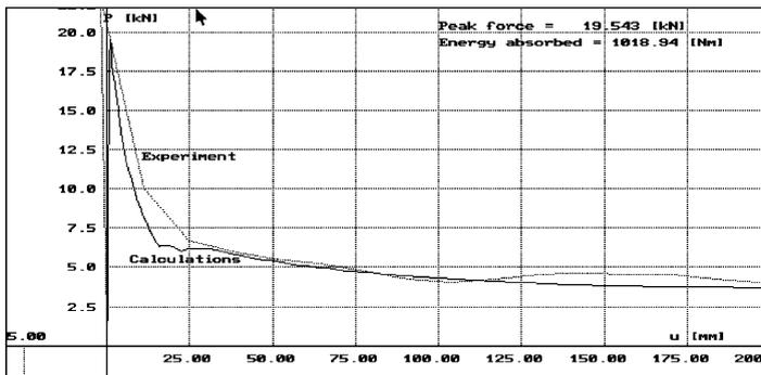
Fig. 12. Comparison of Crash Cad calculations with experimental results. The energy absorption is calculated for the crush of 200 [mm].
