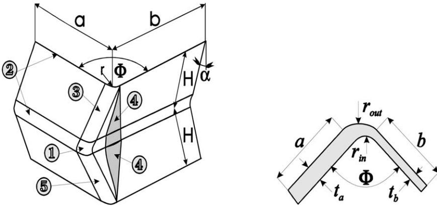
Fig. 2. Idealized deformation mechanisms and cross-sectional dimensions of a Superfolding Element.
