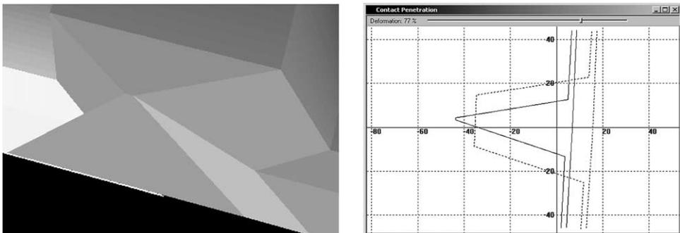
Fig. 8. Predicted collision of propagating plastic hinge lines in a trapezoidal cross-section of rocker panel. The contact occurs at 77% of axial deformation (right picture).
