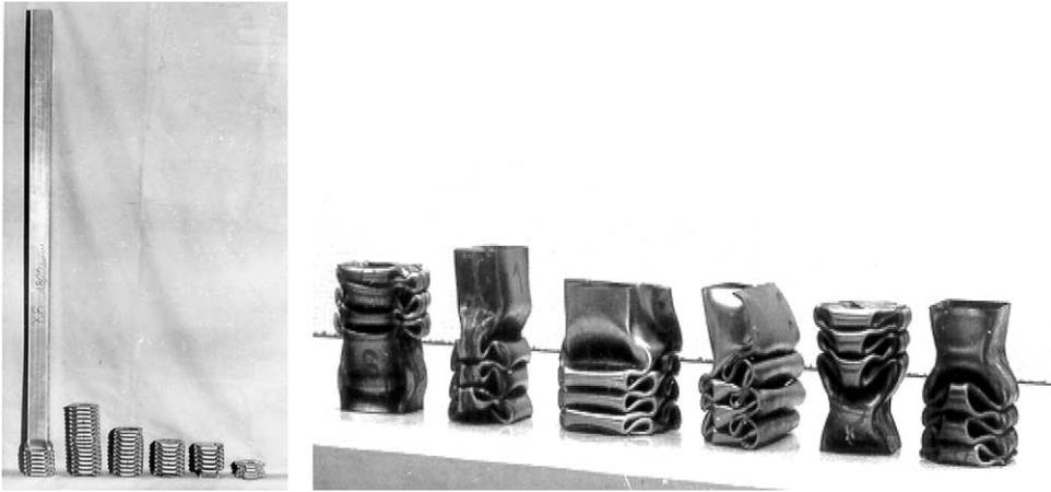
Fig. 6. Progressive folding of properly triggered prismatic members subject to the predominantly axial crash loading.
