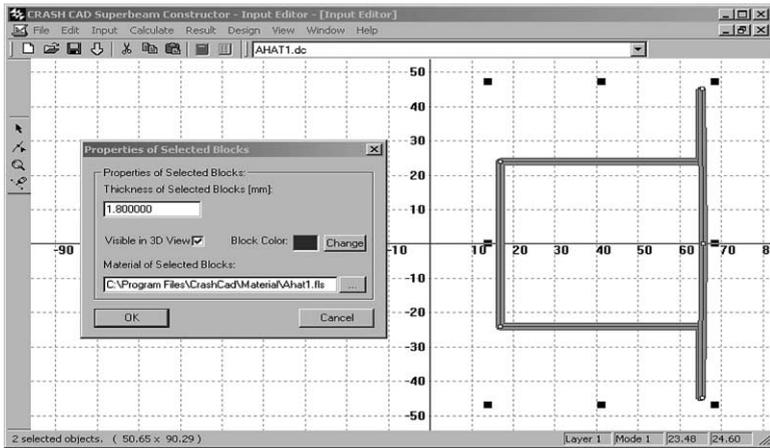
Fig. 7. Input data screen of Crash Cad with a discretized cross-section of a hat member. Only overall dimensions of a section are needed in order to define the Crash Cad input data file.
