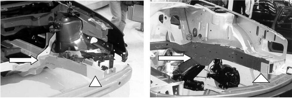
Fig. 10. Energy absorbing structures of the front end of passenger cars. Arrows indicate 'S' frame assemblies. Crash boxes are marked by triangles.
