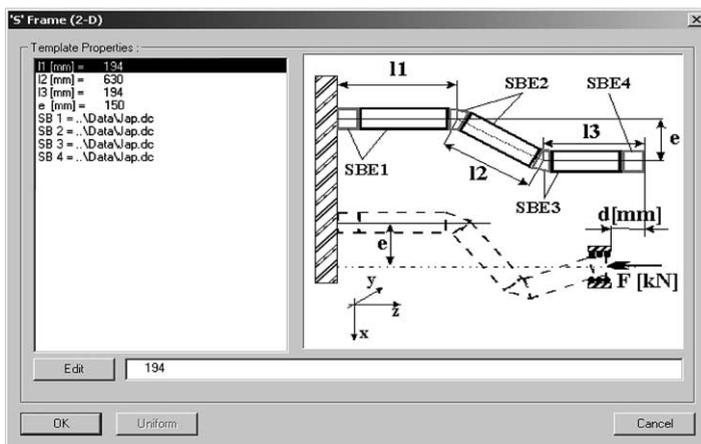
Fig. 11. The input template of 'S' frame model. The whole frame is discretized into four Superbeam Elements. The user is asked to specify the dimensions shown in the figure.
