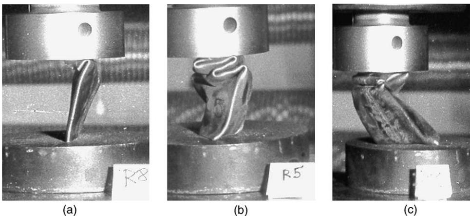
Fig. 4. Global instability of axially compressed prismatic column resulting from incorrect cross-sectional geometry.
