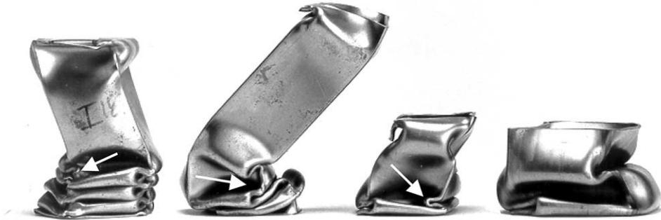
Fig. 5. Global bending of non-triggered square columns resulting from the development of symmetric and 'inverted' folding modes indicated by white arrows
