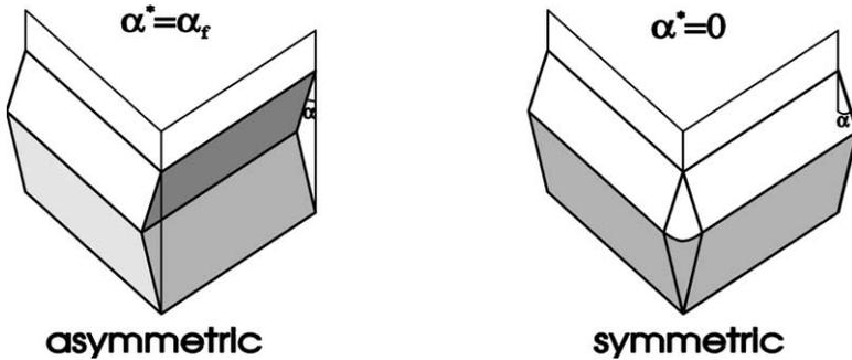
Fig. 3. Two fundamental folding modes of a single Superfolding Element controlled by limit values of the switching parameter  $\alpha^*$ .
