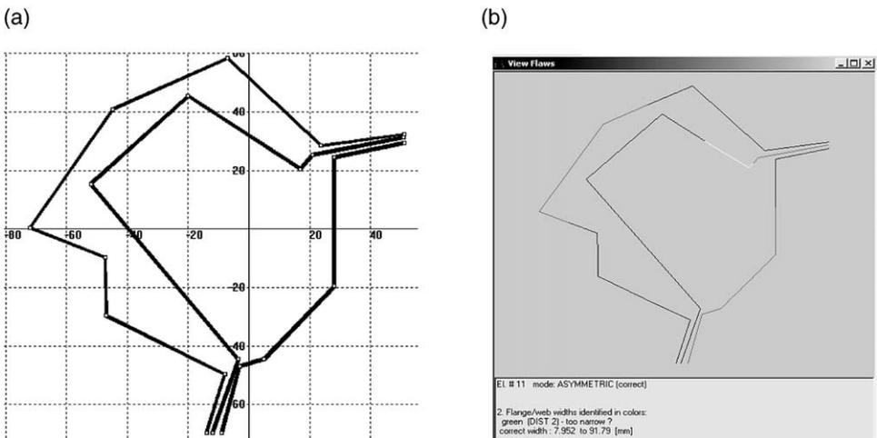
Fig. 9. Cross-section of an early design concept of a longitudinal member (A) and list of design flaws detected during numerical analysis of the folding process (B).
